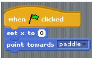
Now that we have set up the initial state of the ball, we need to tell it how to move during the game. We want the ball to keep moving forward, unless it hits a wall or the paddle. To do this, add a forever loop to the bottom of the stack and inside ask the sprite to keep moving 8 steps forward. Try this and see how it works.
